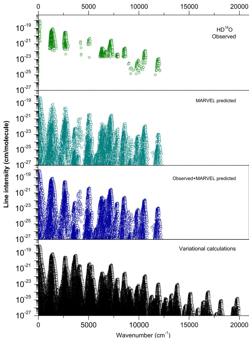
**Fig. 6.** Observed (top panel), MARVEL predicted (second panel), their sum (third panel) transitions based on predictions from variational calculations [116,140] (bottom panel) for  $\text{HD}^{18}\text{O}$ . Calculated line intensities are used in each case.
