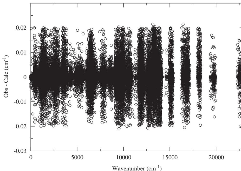
Fig. 3. Differences between the measured transition wavenumbers and those calculated using the MARVEL energy levels derived in this work for HD<sup>16</sup>O.
