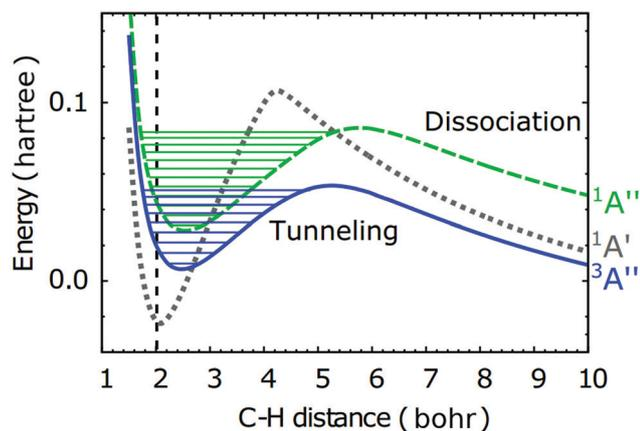
Fig. 15 Calculated potential energy curves along a C–H stretching coordinate of the planar ethylene dication,  $C_2H_4^{2+}$ . The gray dotted line shows the electronic ground state, while the blue solid line and the green dashed line correspond to the first and second electronically excited states, respectively. Horizontal lines represent vibrational states. See ref. 206 for computational details.
